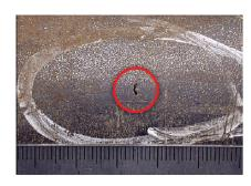
Internal corrosion means localized pitting corrosion (LPC) that causes over 60 % of oil and gas pipeline and facility failures.
