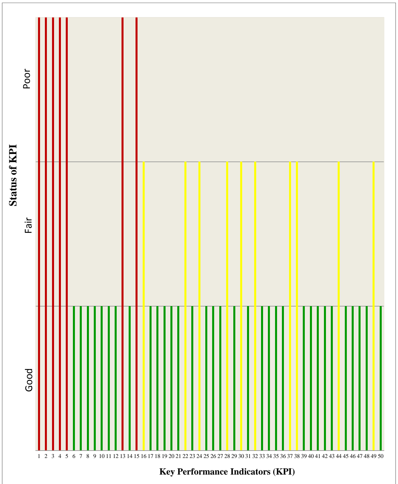
Figure 1. Status of Key Performance Indicators (KPIs) with Respect to Corrosion Control in the Oil Production Pipeline Discussed in this Paper
